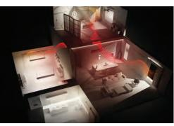
No ducting, fans or power required to circulate the heat. Allows homeowners to design and build their space, completely integrating a fireplace into the décor with true zero clearance to combustible materials.
