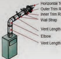
Horizontal Termination Outer Trim Ring Inner Trim Ring Wall Strap Vent Length Elbow
