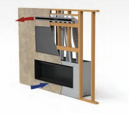
HeatFlo kit option allows heat to be directed above heat sensitive wall hangings.
